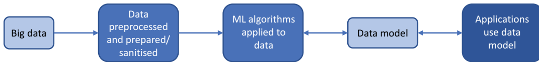
Figure 17.3 Large amounts of raw data are processed and made ready for use. Different preparation techniques and data sanitization may be applied, depending on the raw inputs. Then ML algorithms are applied to the prepared data to build an appropriate data model that reflects the best correlation among all the data points. Different data models may be produced and refined over time. Applications can use the data models on their own data inputs to help guide their decision making and understand patterns.
