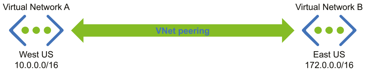
Figure 3.5: Connecting resources in different regions using Global VNet peering
